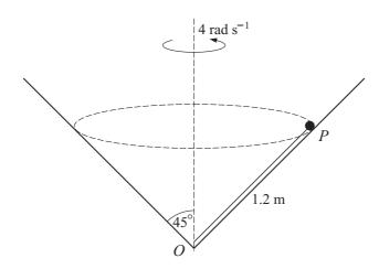
A hollow cone with semi-vertical angle  $45^{\circ}$  is fixed with its axis vertical and its vertex O downwards. A particle P of mass 0.3 kg moves in a horizontal circle on the inner surface of the cone, which is smooth. P is attached to one end of a light inextensible string of length 1.2 m. The other end of the string is attached to the cone at O (see diagram). The string is taut and rotates at a constant angular speed of 4 rad s<sup>-1</sup>.
