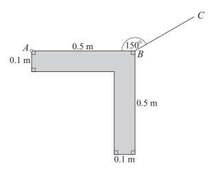
A uniform lamina of weight 9 N has dimensions as shown in the diagram. The lamina is freely hinged to a fixed point at A. A light inextensible string has one end attached to B, and the other end attached to a fixed point C, which is in the same vertical plane as the lamina. The lamina is in equilibrium with AB horizontal and angle  $ABC = 150^{\circ}$ .
